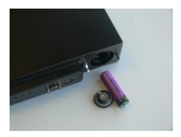
**4.** Insert the new battery, negative end first. The positive end should be visible.
