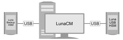
**a.** Install the required client software on the Luna HSM Client workstation and start LunaCM. See "Client Software Required to Perform Backup and Restore Operations" on page 108 for more information.
