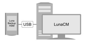
a. Install the required Luna HSM Client software on the workstation, including the **Backup** option. See "Client Software Required to Perform Backup and Restore Operations" on page 108 for details.
